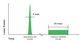
StarWalker's unique VERDE mode delivers 532 nm energy in long millisecond pulses designed for treating superficial vascular lesions.
