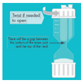
Figure 2: Opening Top Collar
